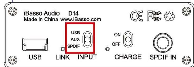
There is an input switch on the rear panel as shown on the above picture. When the switch is on the AUX position, the D14 works as an AMP only, which means it takes analog input from AUX IN/OUT port. When the switch is on the USB position, the D14 takes digital input from the USB port. When changed to the SPDIF position, the D14 takes coaxial or optical digital input from the SPDIF port, provides line out on AUX IN/OUT port and amplified output on the PHONE port.
